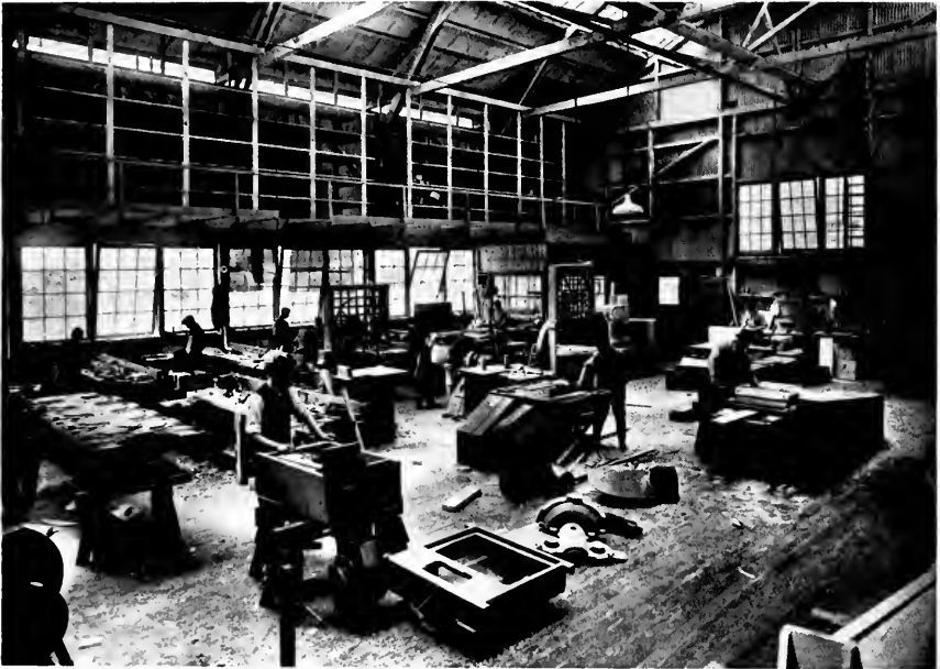
The pattern-shop at the Skandia Pacific Oil Engine Company's plant. Modern motor-driven woodworking tools have been installed here, and in this light, airy shop all Skandia patterns are turned out in duplicate.
